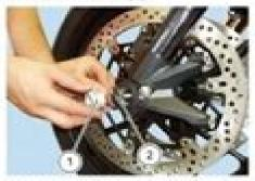
Loosen the axle clamp bolts (B) on the ends of the fork legs...
