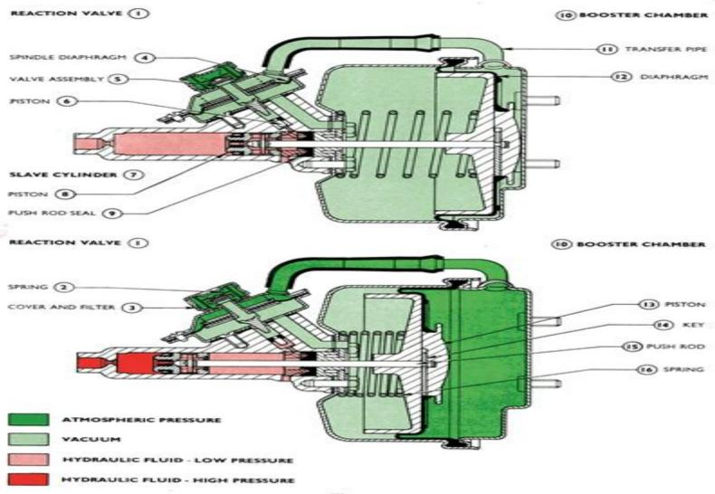
Fig. 24 Servo Unit Operations
