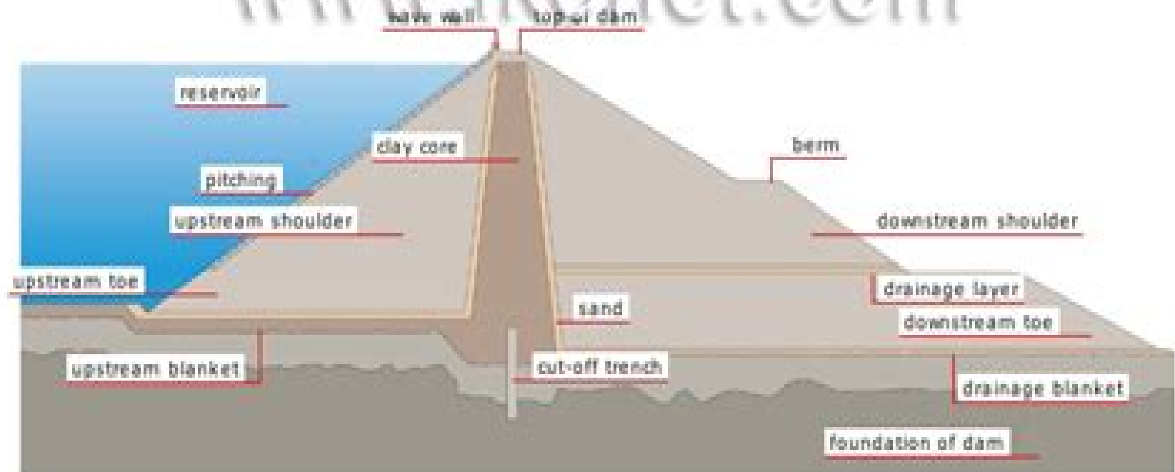
Trans section of an embankment dam
